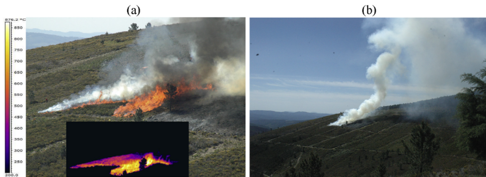
Fig. 6. Combined photo and IR image (colorscale indicating flames temperature) shortly after the point ignition (a) and smoke plume rise during smouldering (b).
