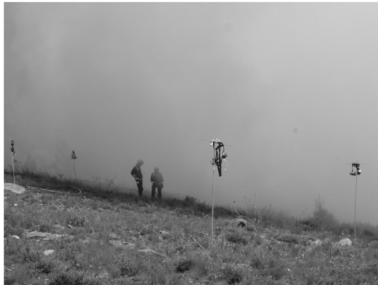
Fig. 2. Mast mounted sensors during the fire experiments (photo taken during the burn of block 2).
