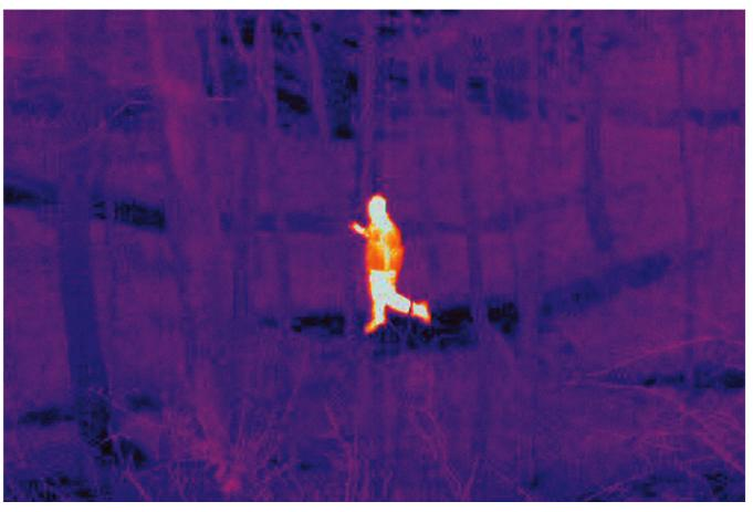
Warmer body parts (red, yellow) emit more infrared energy than cooler (blue) parts Practical Application - Infrared Camera for night-vision: Person detected by infrared energy emissions
