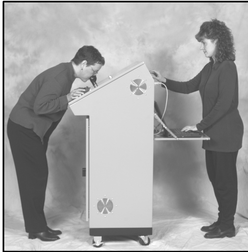
Figure 1. Dynamic dilution olfactometer test (courtesy of St. Croix Sensory).
