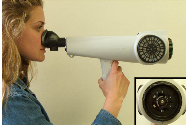
Figure 2. Field olfactometer (courtesy of St. Croix Sensory).
