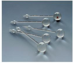
The Little Florentine Thermometer, the first modern thermometer, consisted of a glass tube with a bulb at one end with glass beads welded onto the tube to create a fixed, calibrated reference scale. Previous thermometers had separate scales and were unsealed and thus were affected by air pressure.
