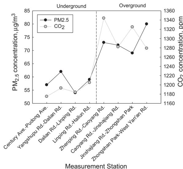
Fig. 5. Average in-carriage  $PM_{2.5}$  and  $CO_2$  concentrations in underground and overground. The Metro Line 4 was used in the measurement.
