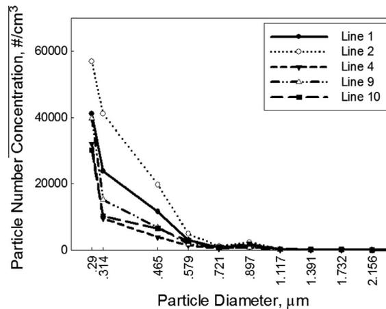
Fig. 4. Particle size distributions measured in different metro carriages.
