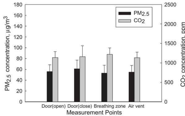
Fig. 7. Average PM<sub>2.5</sub> and CO<sub>2</sub> concentrations in the metro carriage at various measurement points.
