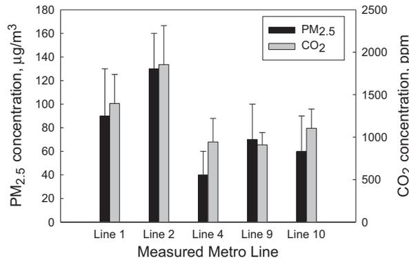
Fig. 3. Average in-carriage PM<sub>2.5</sub> and CO<sub>2</sub> concentrations at five measured metro lines.
