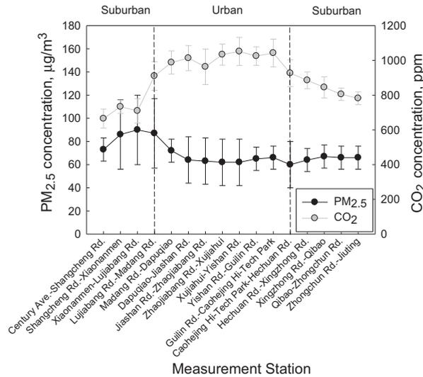
Fig. 6. Average in-carriage PM<sub>2.5</sub> and CO<sub>2</sub> concentrations in urban area and suburban area. The Metro Line 9 was used in the measurement.
