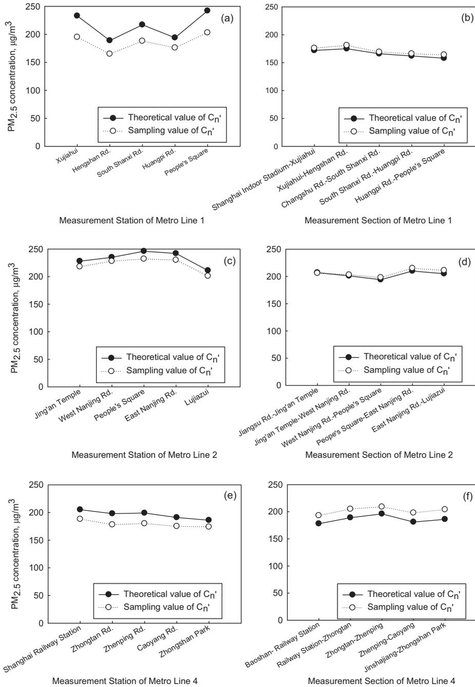
Fig. 9. Comparison between the modeled and the measured in-carriage  $PM_{2.5}$  concentrations when the metro was stopping at the stations: (a), (c), (e) and running between stations: (b), (d), (f). The Metro Line 1, 2, 4 were used in the measurements.
