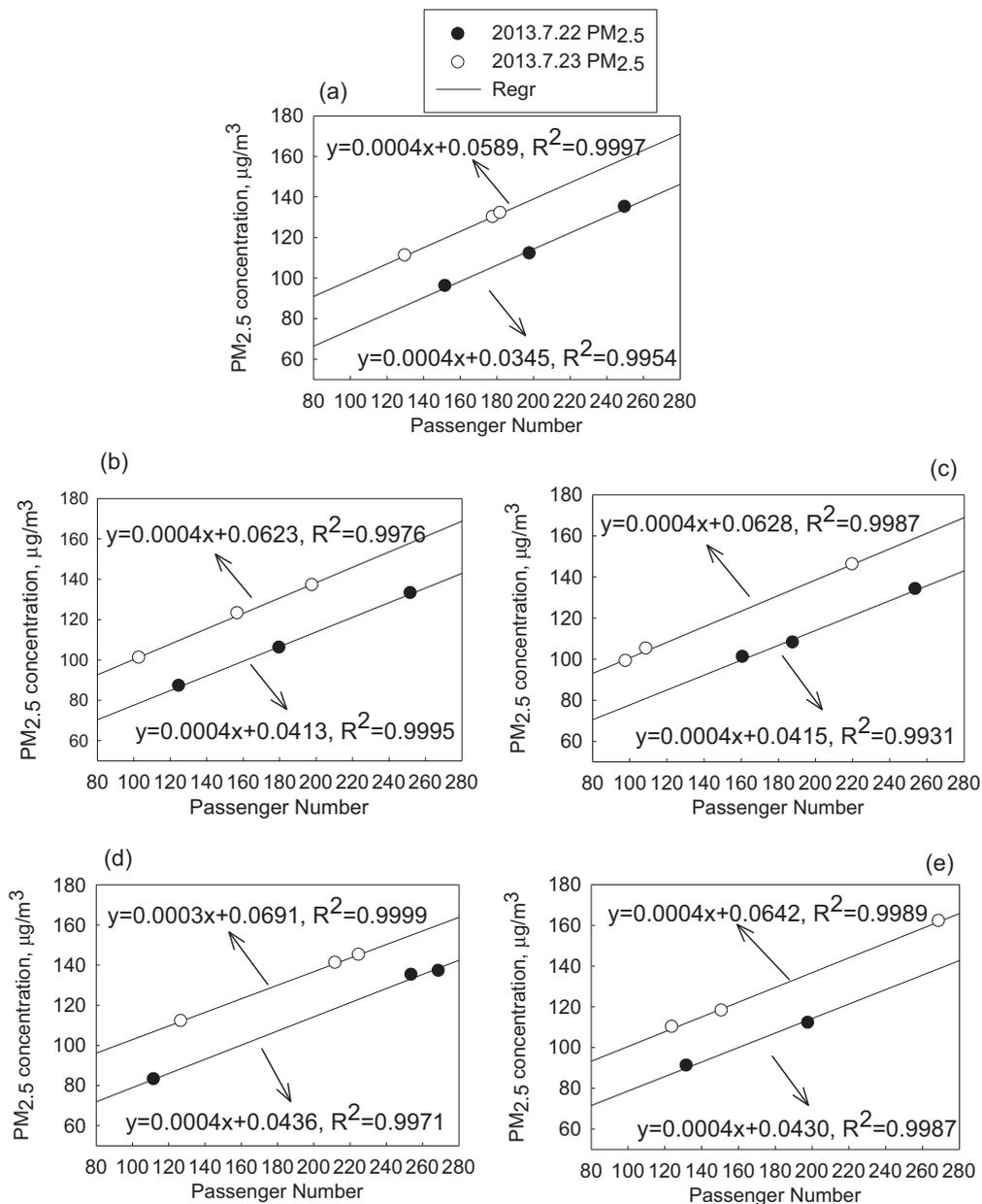
**Fig. 8.** Correlations between the average PM<sub>2.5</sub> concentration and passenger number in the same metro carriage between different stations: (a). Xujiahui to Hengshan Rd., (b). Hengshan Rd. to Changshu Rd., (c). Changshu Rd. to South Shanxi Rd., (d). South Shanxi Rd. to South Huangpi Rd., (e). South Huangpi Rd. to People's Square.
