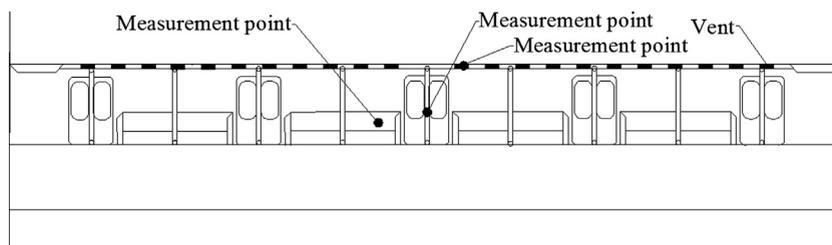
Fig. 1. Schematic diagram of the measurement points inside metro carriages.
