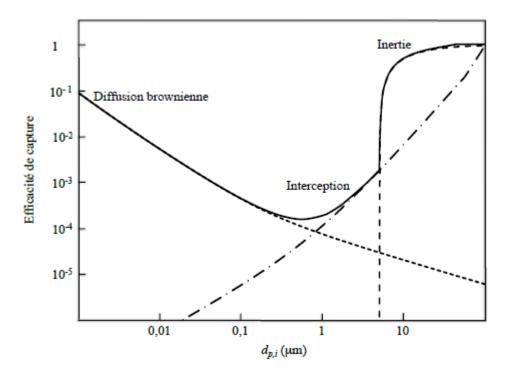
Brownian diffusion dominates for ultrafine particles, i.e. those particles of diameter  $< 0.1 \mu m$ .
